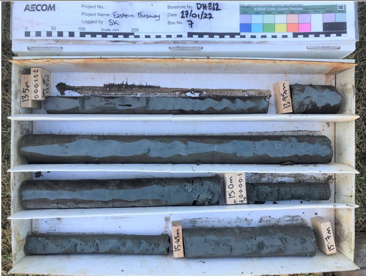
Box: 7 of 12 - Depth: 13.50m to 15.70m of 25.93m Date Drilled 27/01/2022 to 28/01/2022 - Date Photographed: 27/01/2022
