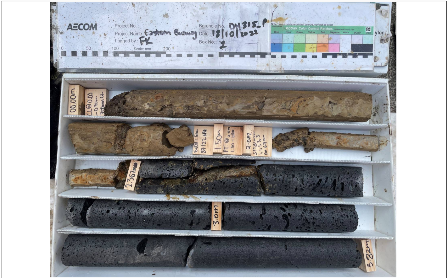
Box: 1 of 11 - Depth: P\DH315_P 0.00m to 3.82m of 31.50m Date Drilled 18/10/2022 to 19/10/2022 - Date Photographed: 18/10/2022
