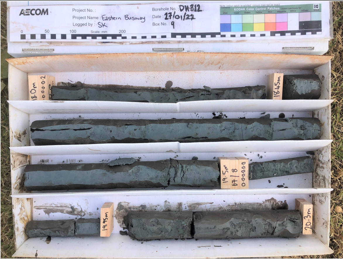
Box: 9 of 12 - Depth: 18.00m to 20.30m of 25.93m Date Drilled 27/01/2022 to 28/01/2022 - Date Photographed: 27/01/2022
