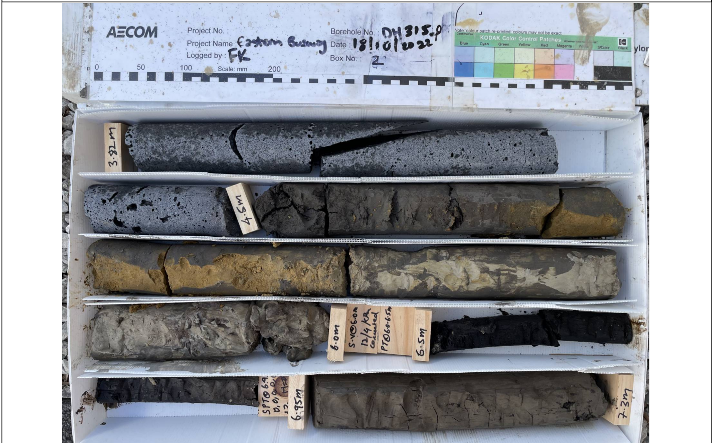
Box: 2 of 11 - Depth: P\DH315_P 3.82m to 7.30m of 31.50m Date Drilled 18/10/2022 to 19/10/2022 - Date Photographed: 18/10/2022
